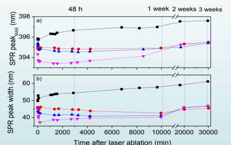
a) SPR peak wavelengths and b) SPR peak width of AgNPs solution obtained by SP and DP-LAL at three representative interpulse delays: ● 10 μs, ▲ 80 μs and ▼ 160 μs respectively, as function of time after laser ablation.
