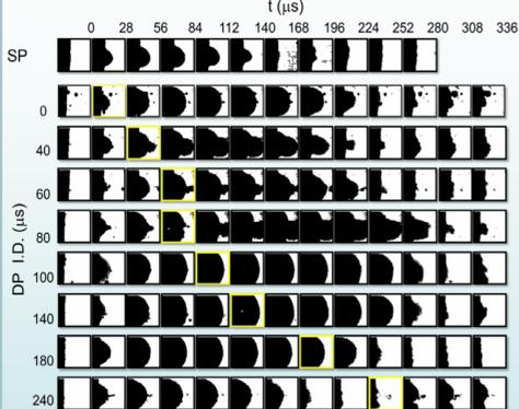
Time-resolved shadowgraph images of bubbles induced by double laser pulses on Ag target in water. The image with yellow square represents the incoming time of the second pulse.
