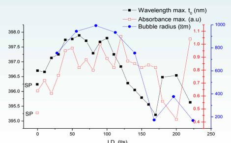
SPR peak wavelength and its absorbance of AgNPs in water as function of interpulse delays prepared by DP-LAL. The first point of graphics corresponds to an AgNPs solution prepared with SP-LAL at the same experimental conditions of DP-LAL. Bubble radius is reported for comparison
