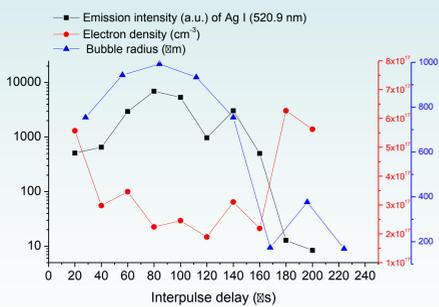
OES measurement of plasma emission produced by the second laser pulse during a DP experiment on Ag target in water. Emission intensity of Ag I spectral line (520.9 nm) and electron number density as function of the delay time between the two laser pulses. The bubble radius temporal evolution
