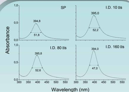
Surface Plasmon Resonance absorption spectra of the AgNPs in water obtained by SP-LAL and by DP-LAL at three representative interpulse delays
